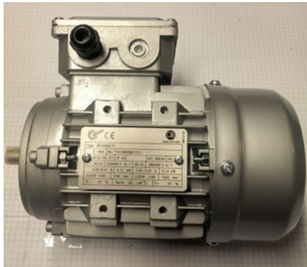
202SK-MS631-4-1 – Electric motor for gear for carriage, 3 phase system, 400V
