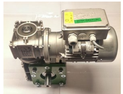
202SK1SI63-F1-2KL – Gearmotor for rotating bar on stirring system, 1 phase, 2 capacitor system (older)
