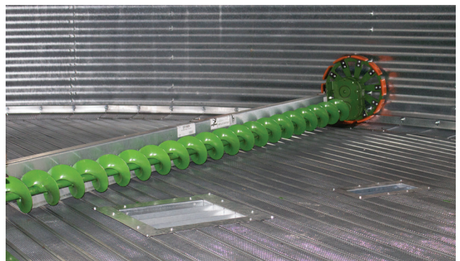
The sweep auger can also be delivered with extra reduced speed on the drive wheel, ratio 16:1 ▼
