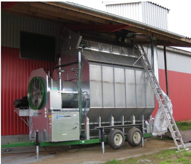
▲ DC 12 mobile dryer with axial fan
