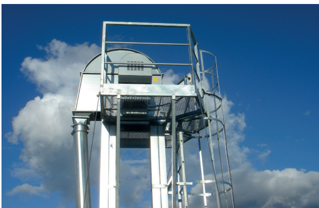
▲ Service platform and ladder with safety cage on elevator pipe for free-standing bucket elevator.
