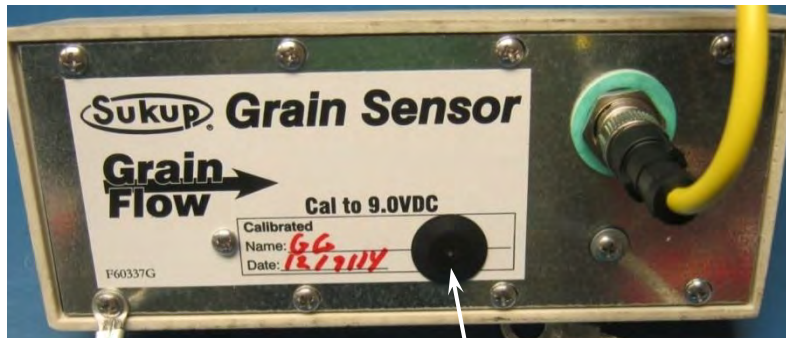
Image 4-15 – Plug over moisture sensor calibration hole
