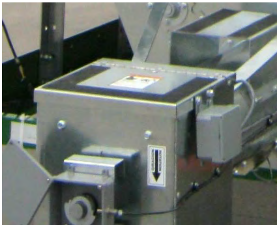
Image 40 – Unload auger service door
