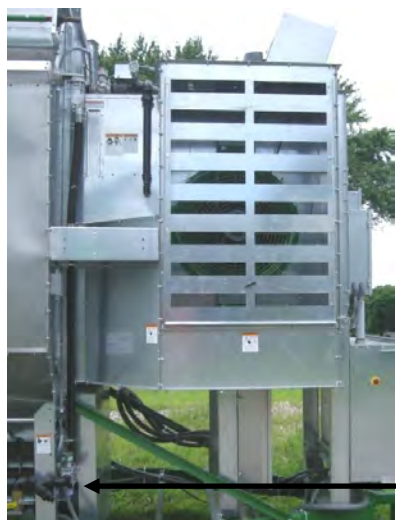
Image 2-2 – Natural gas-fueled centrifugal dryer
