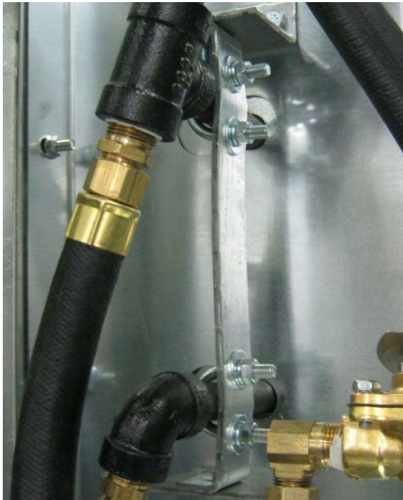
Image 3-1 – Vaporizer adjustment bracket on centrifugal fan dryer
