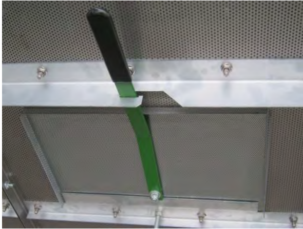
Image 4-36 – Grain column outside cleanout door handle
