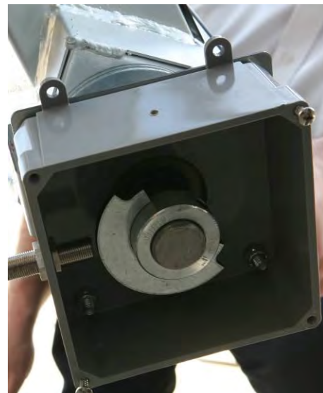
Image 15 – Unload proximity switch mounted on jump auger
