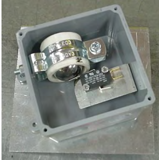
Image 4-3 – Grain discharge chute switch
