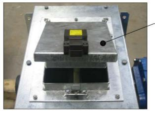
The overfill safety switch shall be installed and checked.
