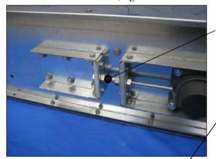
Standard tightening is done in the tight end of the conveyer.
